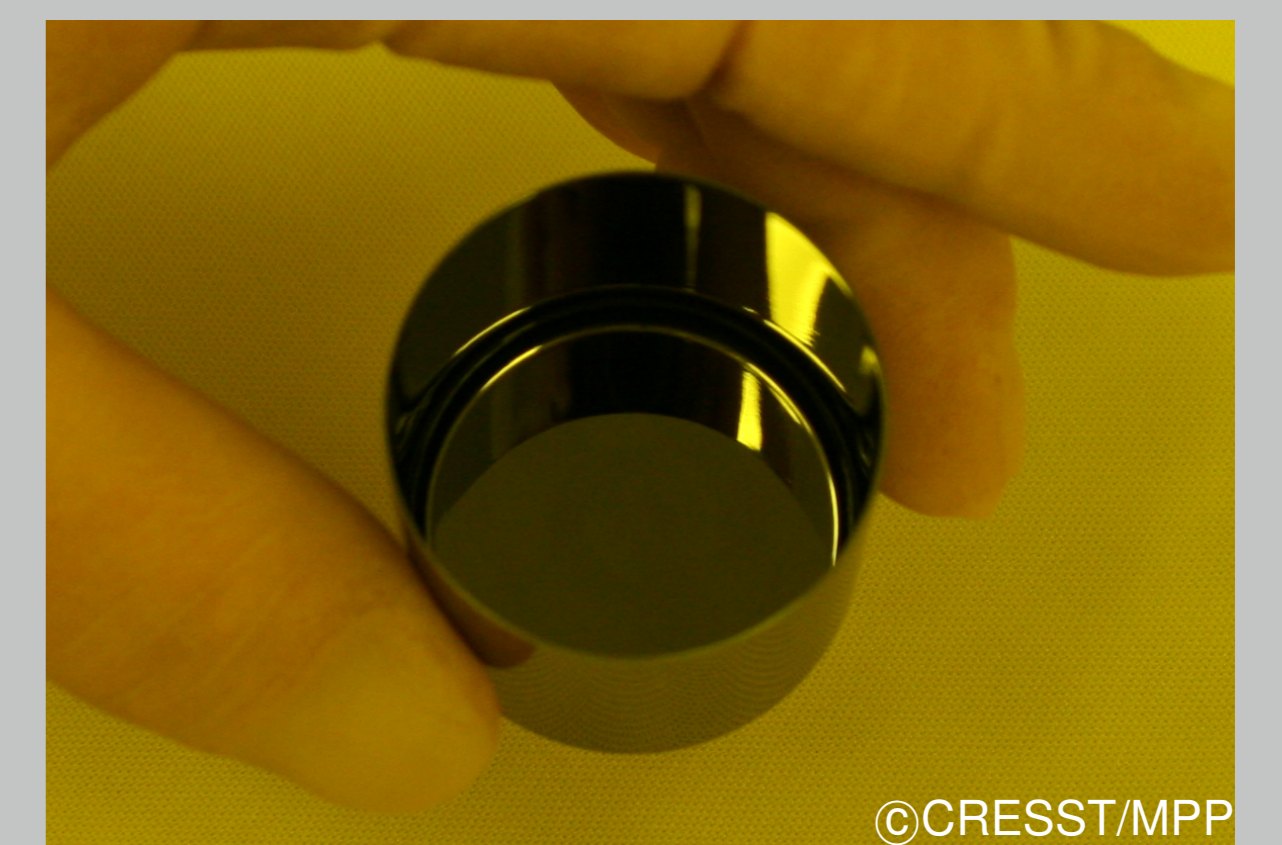
Figure 10: Polished silicon beaker (height 40mm, diameter 40mm, thickness 0.4mm) milled from single crystal material.
