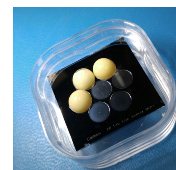
Photograph of a partially populated seating wafer chip with alumina lenslets (lenses are provided by J. Vieira at UIUC)
