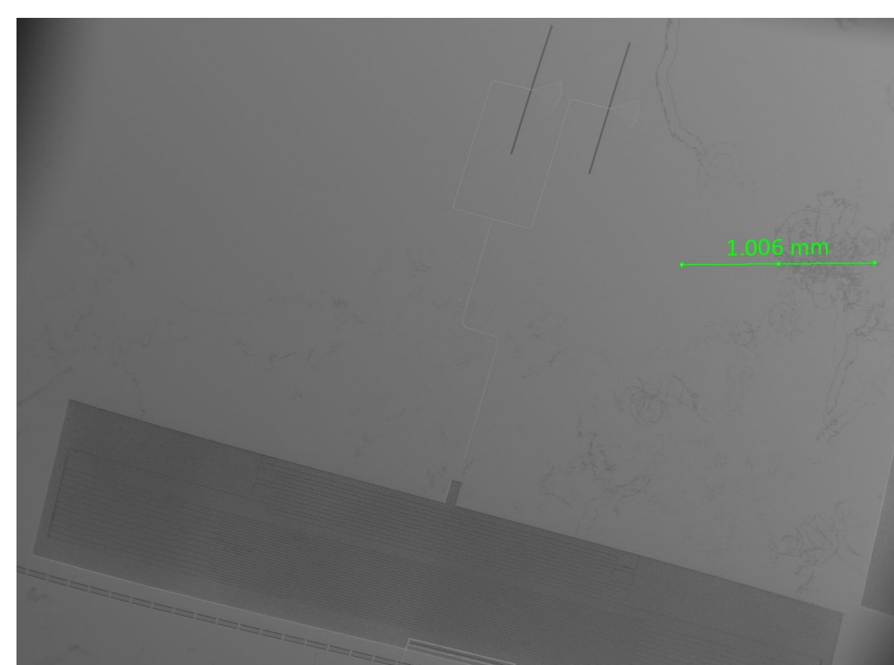
Scanning electron microscope image of an KID with antenna slots.
