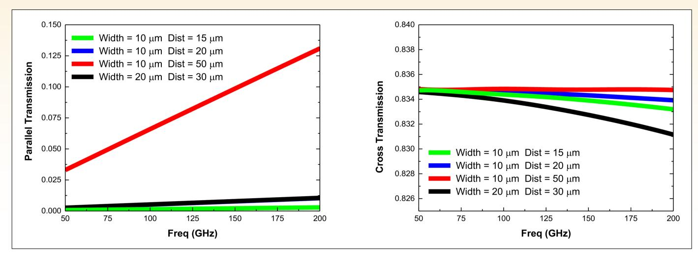
Sonnet simulation of the BiKID structure is shown below. If the spacing between lines is small enough, compared to the resonant frequency wavelength, the wire polarizer acts as an effective ground plane with no influence on the electromagnetic performance.
