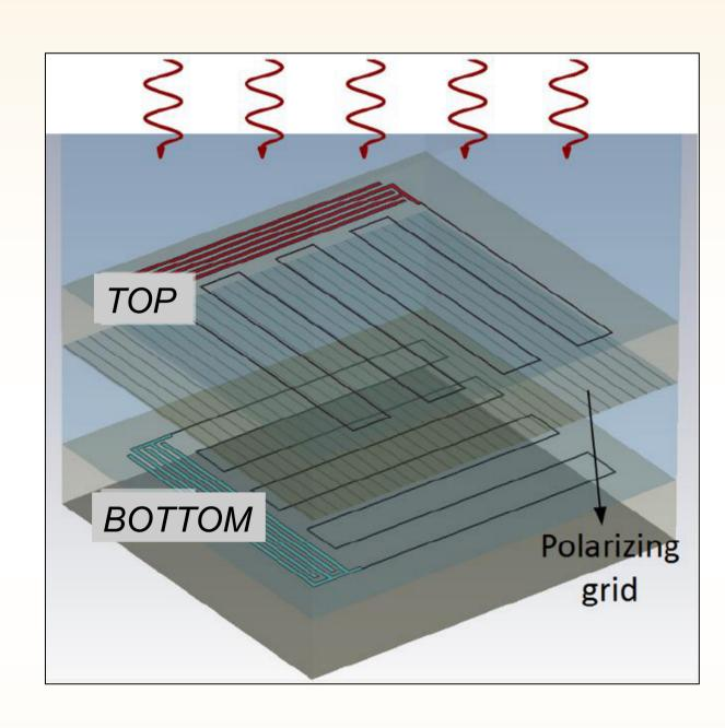
Incoming radiation is coupled from feed-horns to both arrays. Pixels of both arrays (TOP and BOTTOM) are aligned with the center of the feed-horn. A special holder to ensure the alignment has been fabricated.
