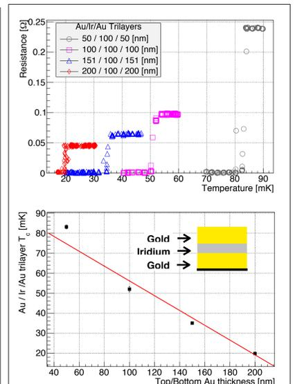
Figure 4. Top) Measured  $T_c$  vs gold thickness on top (or bottom) for Au/Ir/Au trilayers in which all three layers were deposited at room temperature. The iridium thickness is 100 nm for all samples. The same amount of gold was deposited on top and bottom of the iridium. Bottom) Resistance vs temperature data for each Au/Ir/Au trilayer. A bias current of 31.6 A was used.
