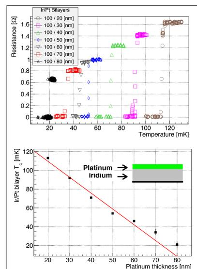
Figure 3. Top) Measurements of the  $T_c$  suppression in Ir/Pt bilayers in which both the iridium (100 nm) and platinum (20-70 nm) layers were deposited at room temperature. A bias current of 3.16 A was used and the uncertainty in the  $T_c$  measurement includes the difference between scans increasing or decreasing in temperature. Bottom) Resistance vs temperature data for Ir/Pt bilayers and from which  $T_c$  was obtained.
