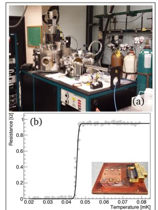
Figure 2 (a) Sputtering chamber at ANL. (b) Resistance vs temperature data and fit for an Ir/Pt bilayer (Ir=100 nm and Pt=60 nm).
