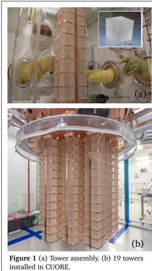
Figure 1 (a) Tower assembly. (b) 19 towers installed in CUORE.
