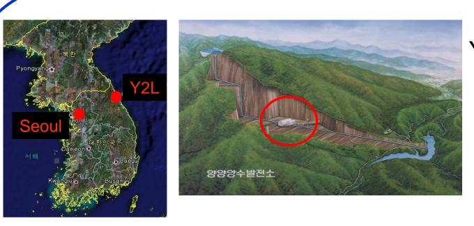
YangYang Underground Laboratory (Y2L) Located in a tunnel of the Yangyang pumped storage power plant (Korea) Minimum vertical depth : 700 m Access to the lab by car : 2 km
