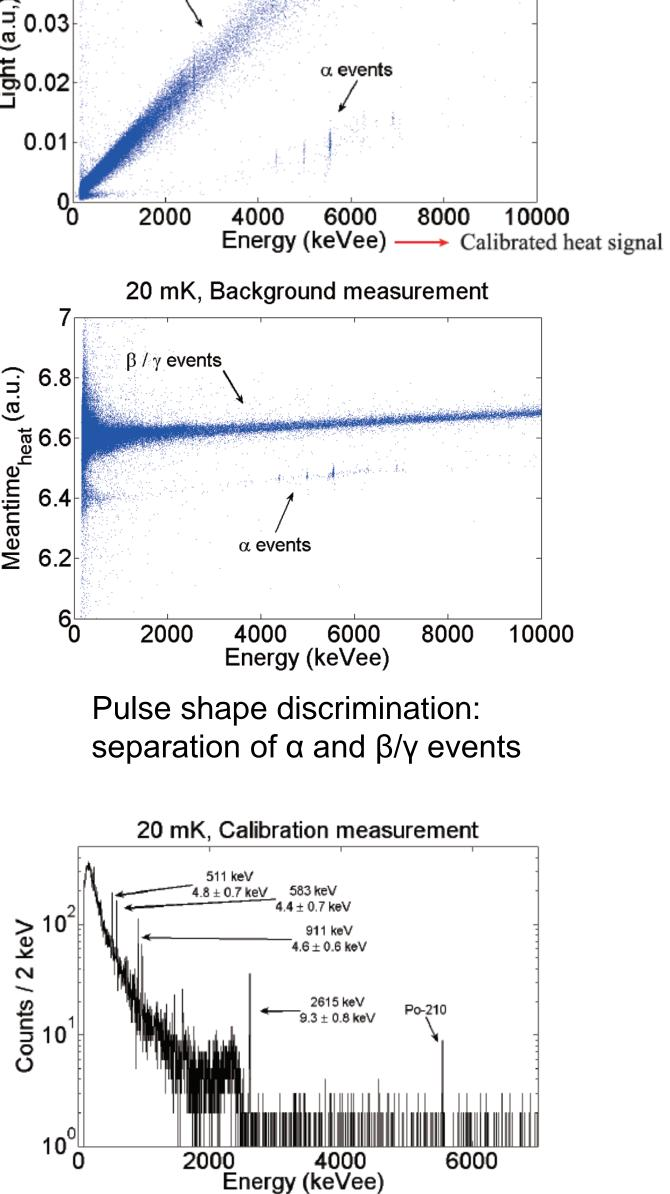
Energy spectrum obtained with an external <sup>232</sup>Th source ΔE<sub>FWHM</sub> ≈ 9 keV @ 2.6 MeV
