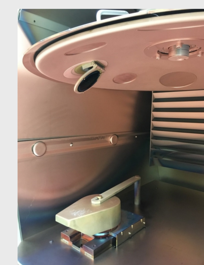
Tilted position of the wafer in the evaporator
