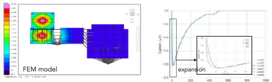
Fig. 4. FEM model of the model TES microcalorimeter (left) and the pulse shapes when an axion is converted at different positions of the <sup>57</sup>Fe converter (right).
