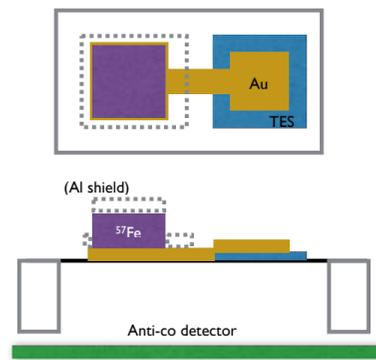
Fig. 3. Model TES microcalorimeter
