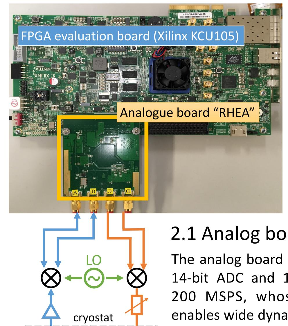
Readout electronics for MKIDs consists of: (i) Carrier wave creation (ii) Return wave
