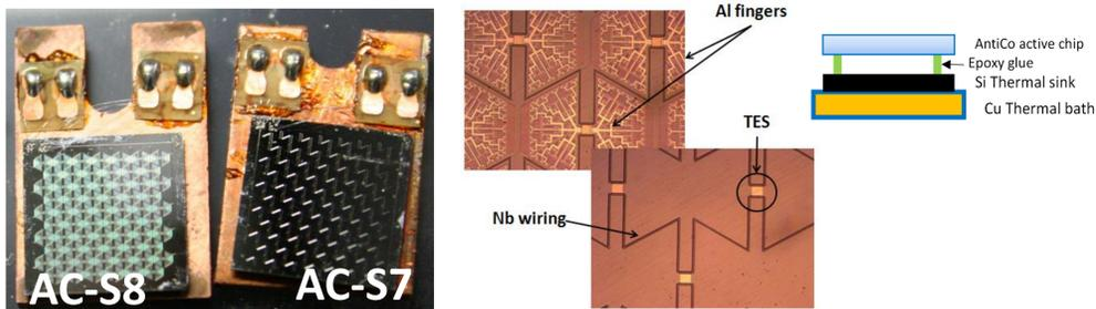
AC-S8 has in addition a **network of Al-fingers** directly connected to the TESes to investigate the feasibility of further improve the Athermal collecting efficiency.
