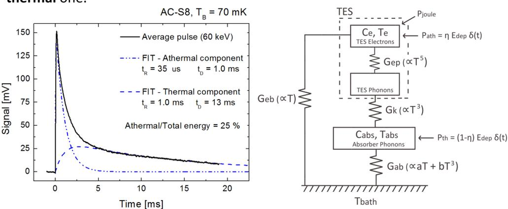
This dynamic could be explained with the thermal model illustrated in the picture, **where a fraction  $\eta$  of the energy deposited by a particle is injected directly on the TES** through the athermal phonon population.
