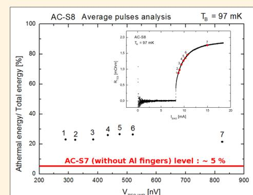
From the average pulse we have found that for AC-S8 the ratio between the athermal and the total (athermal + thermal) energy associated to the pulses is  $\sim 25\%$ , about a factor 4 above the AC-S7 one (see D'Andrea et al. 2017, DOI: 10.1117/12.2231412). This is an evidence of the **increase of the athermals collection efficiency due to the Al finger network**.
