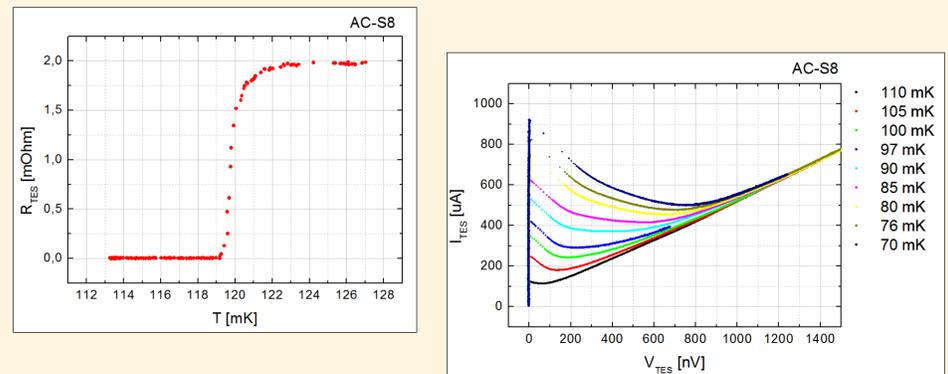
→ The critical temperature ( $T_c \sim 120$  mK) and the narrow transition ( $\Delta T_{10-90\%} \sim 2$  mK) demonstrate the **uniformity of the TES network**.
