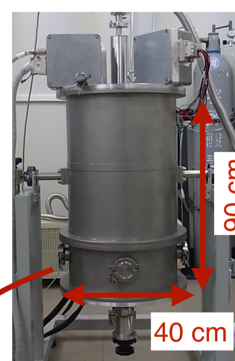
fig4. Appearance of cryostat
