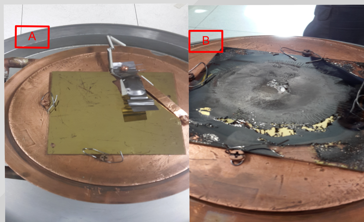
A) Quartz substrate coated with gold before Ho evaporation B) Quartz substrate after Holmium evaporation
