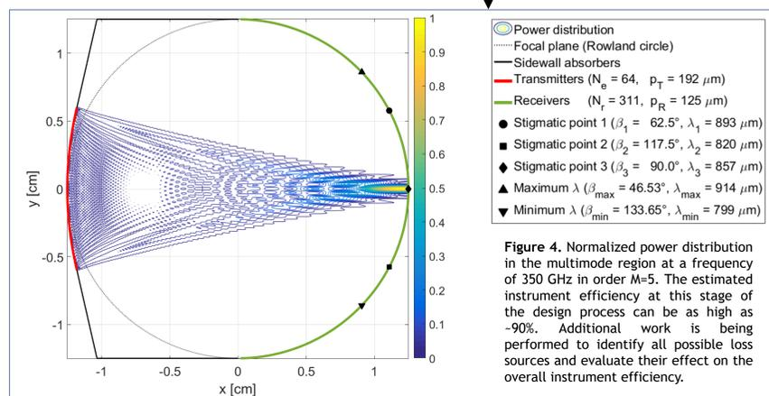
**Figure 4.** Normalized power distribution in the multimode region at a frequency of 350 GHz in order  $M=5$ . The estimated instrument efficiency at this stage of the design process can be as high as  $\sim 90\%$ . Additional work is being performed to identify all possible loss sources and evaluate their effect on the overall instrument efficiency.
