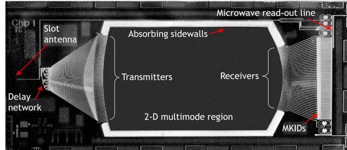
**Figure 2.** A test version with resolving power equal to 64 was designed [8], built and tested at NASA GSFC. The fabrication process developed [9 and Fig. 7] was employed to build several prototypes. The successful instrument optical performance tests have enabled us to demonstrate the  $\mu$ -Spec technology [10].
