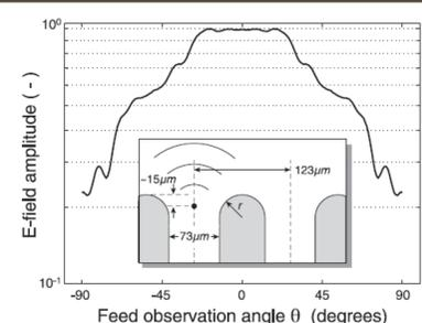
**Figure 6** (Adapted from [8]). (Left) Computed feed horn angular response at 430 GHz. The response of an emitting feed is evaluated in the far field ( $r=6\lambda = 438 \mu\text{m}$ ) and normalized to the magnitude of the E field at  $0^\circ$ . The feed array geometry is provided in the figure insert. The feed's phase center is indicated by a black filled circle.
