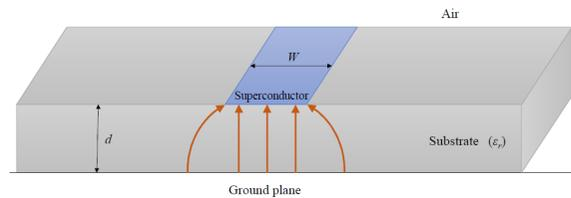
**Figure 3.** Geometry of a microstrip transmission line. In orange are the electric field lines indicating their dominant modal symmetry [11]. This structure can be fabricated by photolithographic processes and integrated with other active or passive microwave devices. It is mass producible and enables reducing the instrument size by a factor of the medium's effective index.
