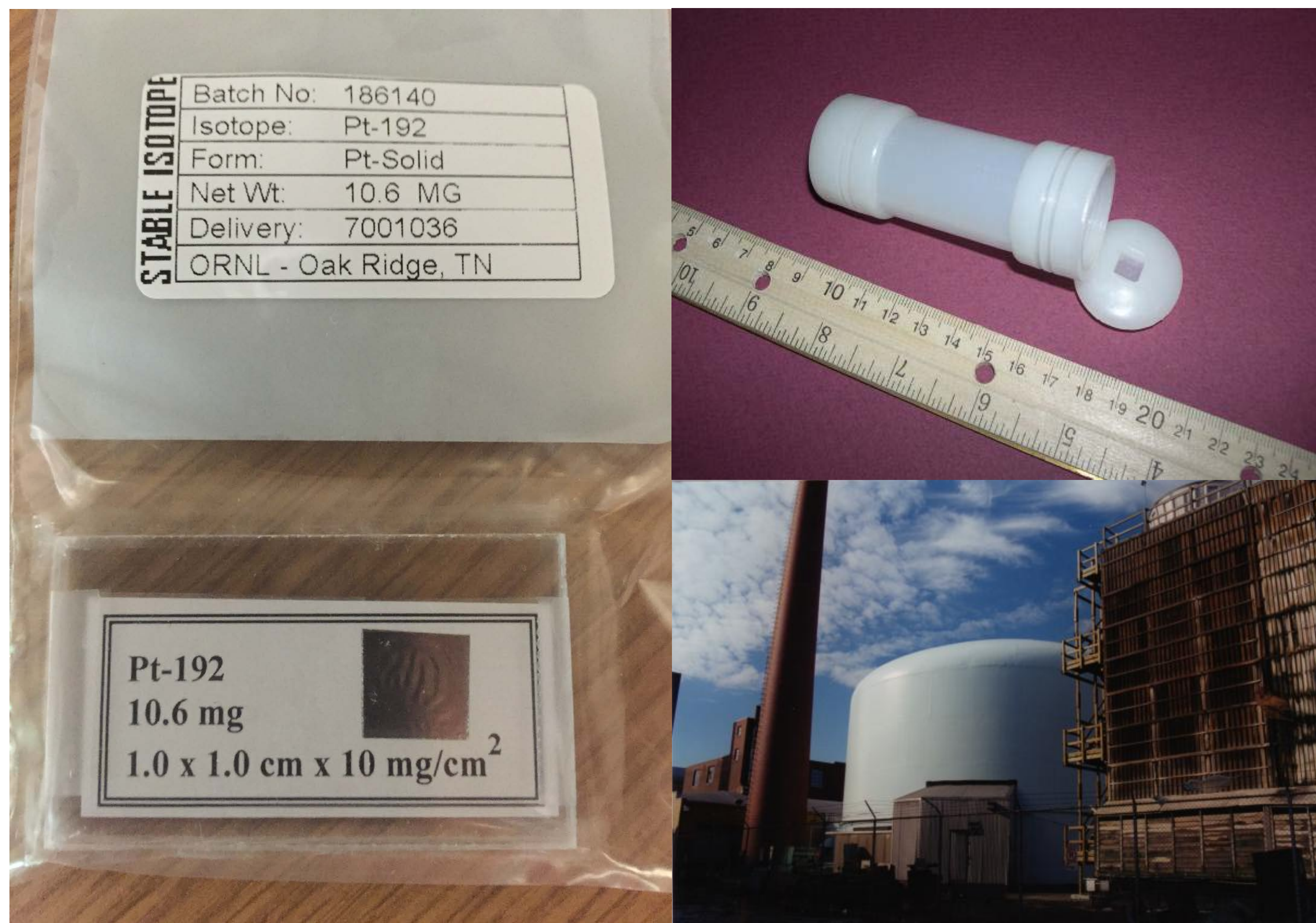
Figure 1. The ^{192}\text{Pt} -enriched Pt foil (left), placed within a polyethylene tube (upper right), was irradiated at the MIT reactor (lower right), exposing it to a high thermal flux to create ^{193}\text{Pt} .
