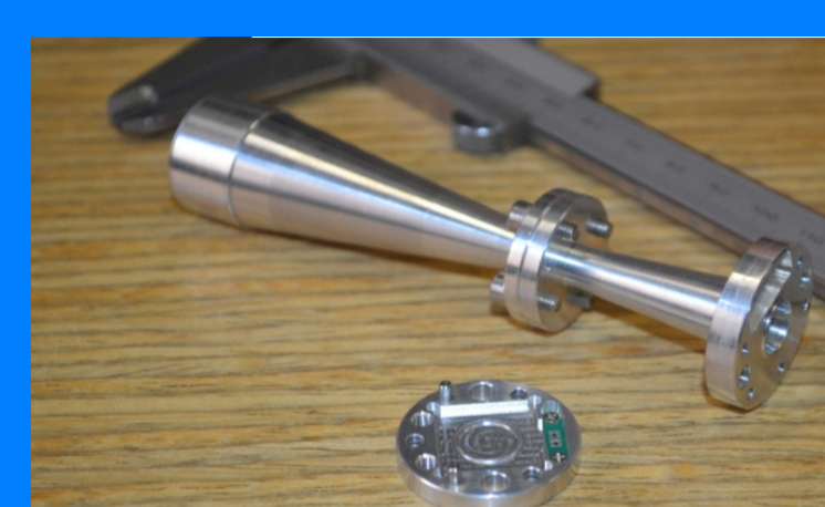
Lower right: one of the multimode horns to be mounted on the focal plane. The dismounted backshot shows the housing for the spiderweb TES.
