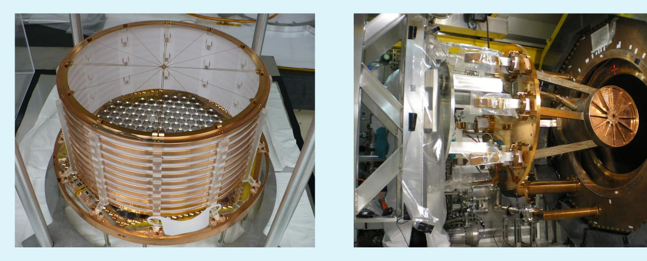
Because different kinds of particle interactions result in different ratios of scintillation to ionization, liquid xenon detectors have an excellent particle discrimination capability for background rejection.
