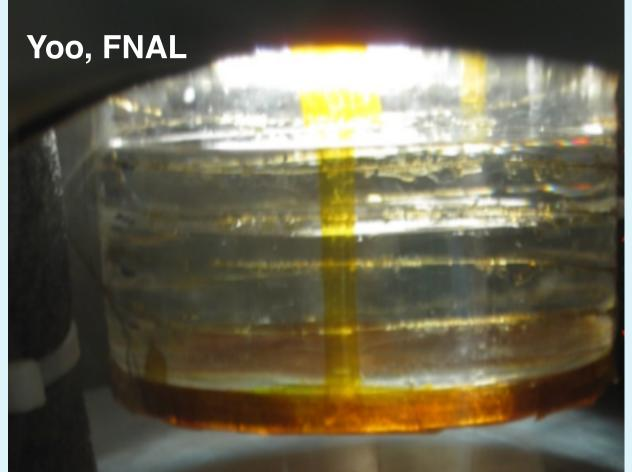
A group at Fermilab has built on work done at Syracuse University using a cryobath method to produced large (~1 kg) solid xenon crystals at a temperature of ~160 K [8]. This work demonstrates the feasibility of growing large, transparent solid xenon crystals, although it is not well-suited for bolometer growth. The group has demonstrated ionization collection in solid xenon at high
