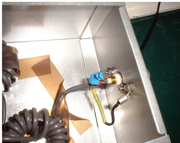
Fig. 4.15: A picture of the condensers in the common-mode filter box.
