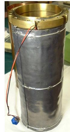
Fig. 4.12: The superconducting magnetic shield made of lead covering the IVC.
