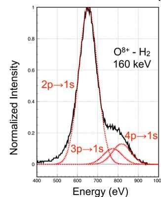
Result of window-less Si(Li) detector [5]. The spectrum show the 2p→1s line is the strongest, and suggests existence of the 3p→1s and 4p→1s lines.
